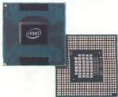
The Intel Core 2 Duo processor; other chip manufacturers are AMD and Motorola
