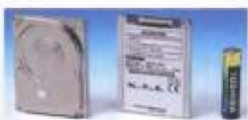
Toshiba's 1.8" hard drive; mini hard drives are used in small gadgets, such as PDAs and wristwatches
