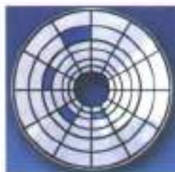
In a fragmented disk, a file is stored in non-continuous sectors.
