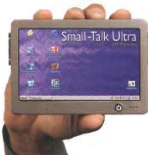
Small-Talk Ultra, a talking computer from GW Micro, which includes Window-Eyes – a screen reader for the blind
