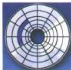
In a defragmented disk, a file is stored in neighbouring sectors.
